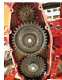
Rugged Gear Drive Transmission
