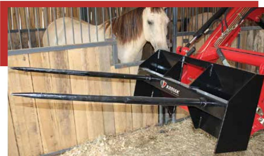
Skid-steer/quick attach front single and double bale spears are designed to fit quick attach loaders and skid steer loaders. These units have a capacity of 2,500 LB on the single spear and 3,000 LB on the double spear. With today's heavy bales, either of these well built spears are a must for any round bale operation.
