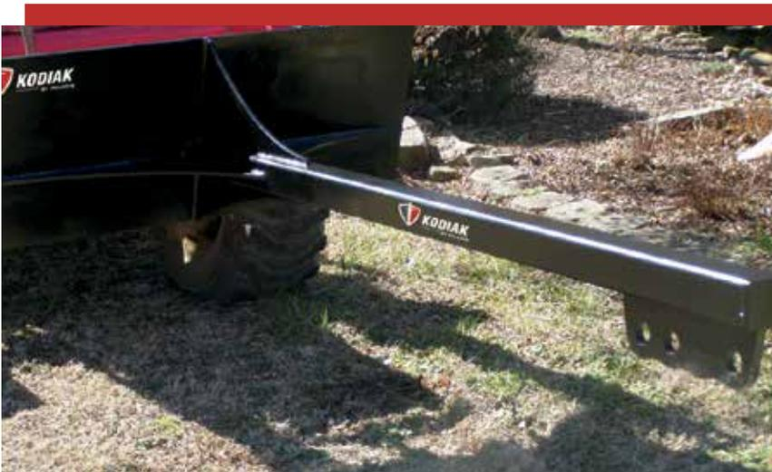
The skid-steer/quick attach tree boom attachments can convert a front loader, or skid-steer, into a boom loader. This unit has a 1,500 LB lifting capacity (depending on loader capacity), which has a multitude of uses around the farm or construction site.
