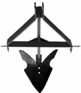
This potato plow is versatile tool that has more than just digging spuds. When set at the proper depth, this implement can also be used for laying off rows in a vegetable garden or going light ditch work to improve drainage. This unit is compatible with tractors up to 40 HP.
