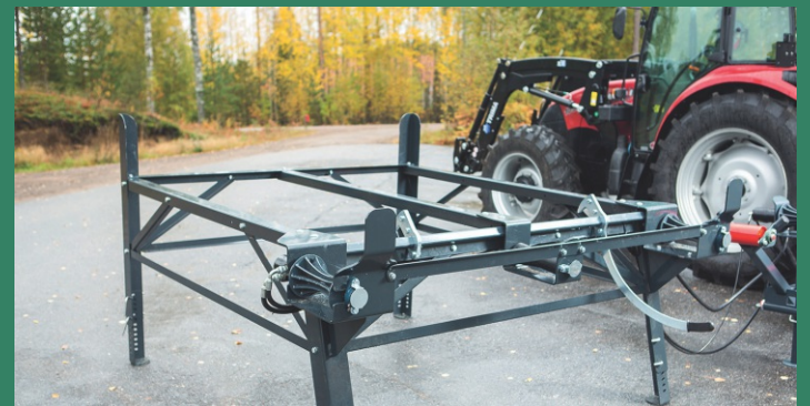
The log deck facilitates and accelerates the feeding of logs into the machine
