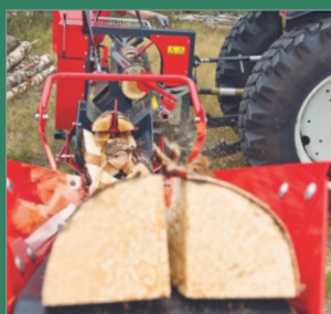
Hydraulic feeding roller makes log feeding easy and light
