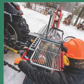
The log deck facilitates and accelerates the feeding of logs into the machine
