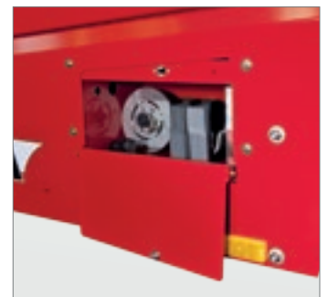
Integrated tool box in the drawbar
