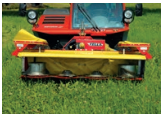
Four mower discs for symmetrically central running
