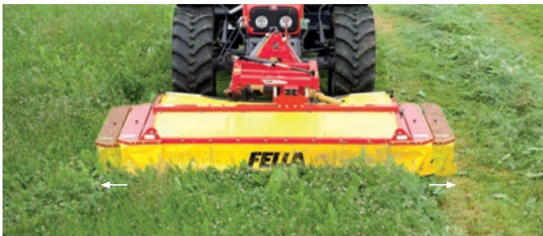
SM 260 FP-S: steplessly hydraulically adjustable sideways (approx. 20 cm on either side)
