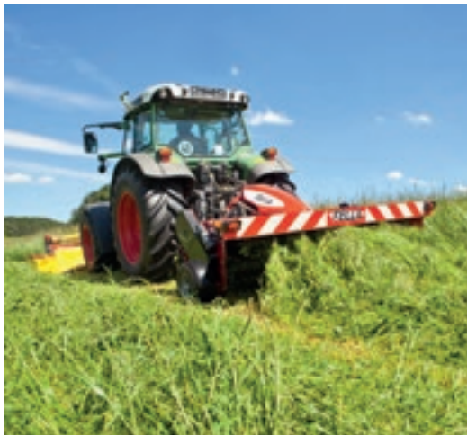
KC 285 D – forage can be deposited across the entire width (left) or in a narrow swath (right)
