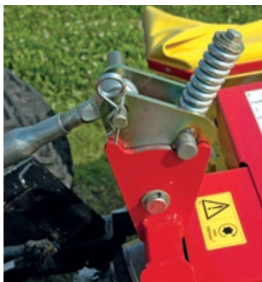
Spring-loaded impact guard system
