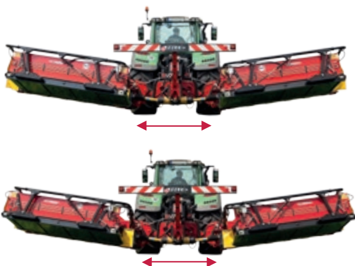
Hydraulic lateral movement of the conveyor belt
