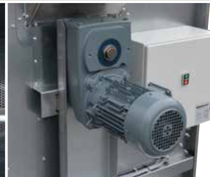
Gear with parallel shaft's makes it easy to turn drum by hand, makes screen change easier.
