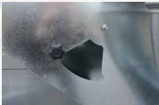
Access door for easy collection of grain sample after cleaning.
