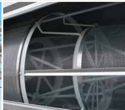
Two layers, one layer for oversize impurities, a second layer for under-size impurities.
