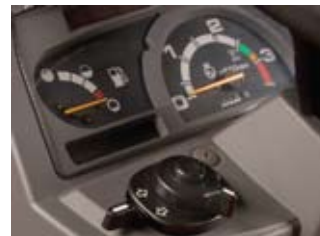
Analog Instrument Panel: Automotive-style instrumentation panel design makes it easier to keep an eye on major operating systems such as a tachometer, fuel gauge and engine coolant gauge.
