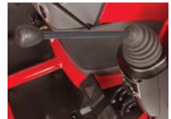
Factory Joystick: Standard on GC2410, GC2600 and GC2610 and optional on the GC2400.
