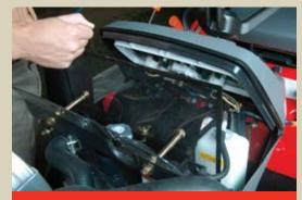
A removable, easy-to-clean screen protects the radiator from dirt and other debris.
