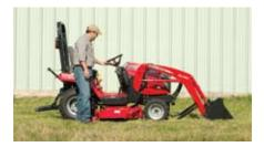
Step 2 Next, use the tractor hydraulics to raise the loader frame out of the mounts.
