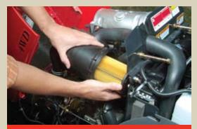
It's easy to check the engine air cleaner, located on the left side of the engine just under the hood.
