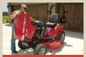
The flip-up hood provides quick and easy access to the engine compartment.
