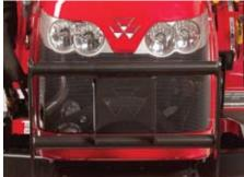
**Grill Guard** Along with providing added protection, the rugged grill guard can be used to carry front weights for added stability and traction.
