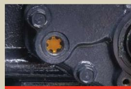
Keep an eye on the hydraulic oil level by simply checking the sight glass.
