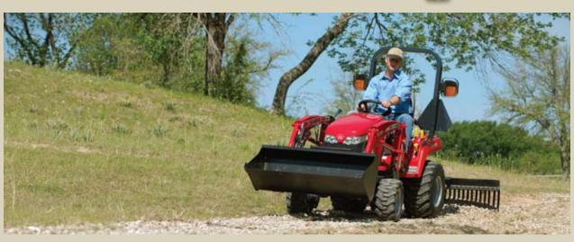
Another big tractor feature you'll find on every GC Series sub-compact is the Category I three-point hitch. Just couple it to the properly matched finish mower, rotary tiller, landscape rake, box blade, grader blade, posthole digger or fertilizer spreader and there's almost nothing you can't do. Plus, if you have multiple jobs on your list, switching out implements couldn't be easier.
